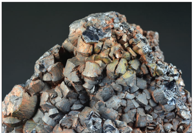
Figure 59. Curvilinear crystals of lithiophorite, field of view 8.2 cm, Gloucester mine. Bruce Cairncross specimen and photo.
